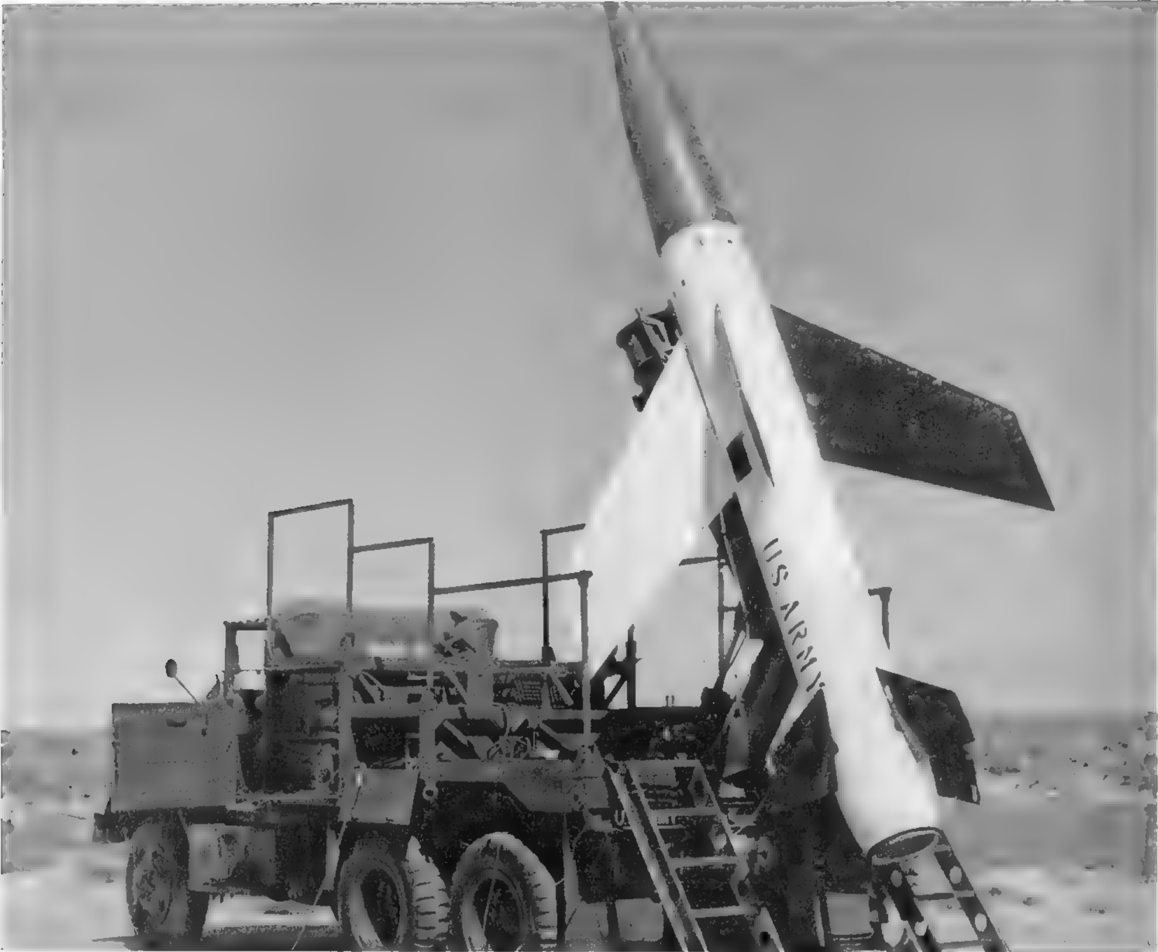
The operational version of the LaCrosse launcher was the M398. It mounted a more sophisticated helical-railed launcher on the dual-wheel M45 chassis. (U.S. Army photo)
